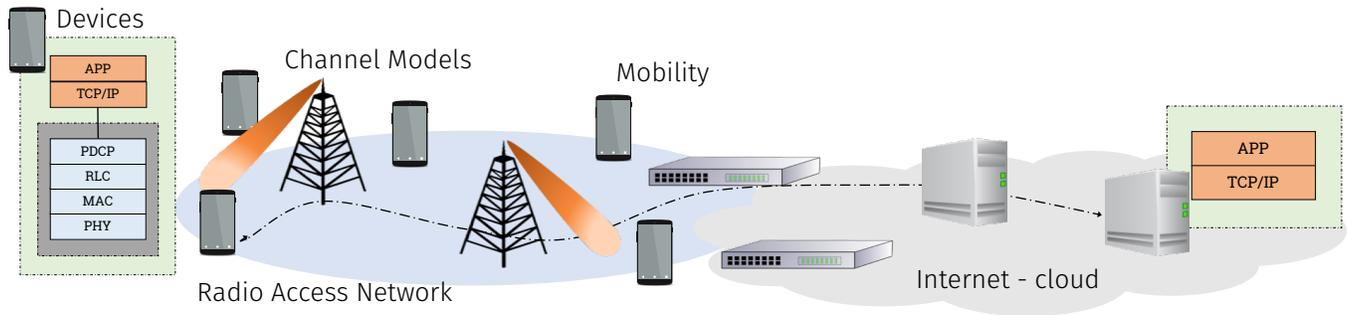
Figure 1: Elements Involved in the End-to-end Simulation of a Cellular Network
